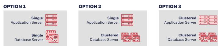
The availability requirements for development and test environments are typically low, and these environments do not need to have a high availability configuration from a cost perspective. The production environment needs to have a high availability.
