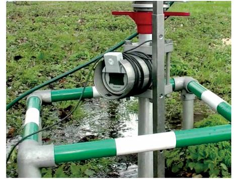
The Q4000 water meter forms part of the total standpipe solution.
