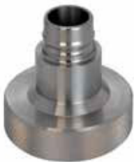
TS 55000 - Used to connect all HERMetric units with 1Inch quick connect coupling to valves with UNF 2 1/2 Inch connection.
