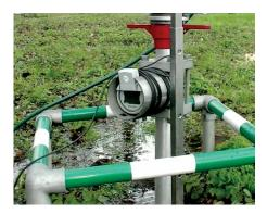
The Q4000 water meter forms part of the total standpipe solution.
